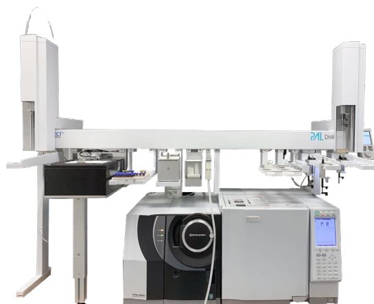
Figure 1: CHRONECT Workstation MCPD with Bruker GC-TQ MS.
